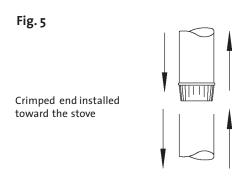
This prevents any amount of condensed or liquid creosote from running down the outside of the pipe or the stove top. All joints, including the flue collar connection must be secured with three sheet metal screws to ensure that the sections do not separate.
